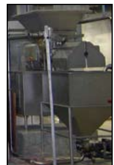
Hopper connected to a Rectangular Flange PD Pump.
